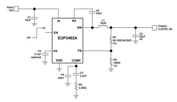
Figure 1. 12V to 3.3V/5V Application Circuit
