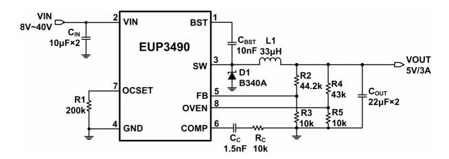
Figure 1. 5V Application Circuit
