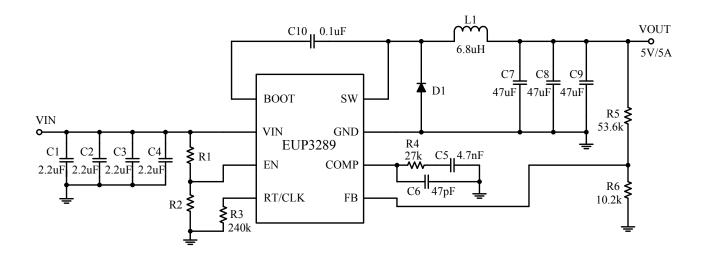
Figure 1. Application Circuit
