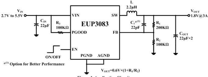
Figure 1. Application Circuit
